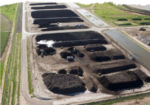
Windrow composting, images courtesy of Jeffries Group.
